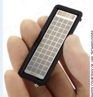
The gene chip was customized using OpenArray technology on the Life Technologies QuantStudio system.
